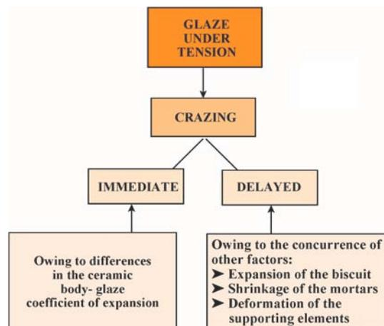
This defect was present in the manufacture of tiles with lead silicate-based glazes, with coefficients of linear thermal expansion exceeding those of the biscuit, affecting both (white body) earthenware tiles and (red body) majolica tiles. In the European standard of 1982, crazing resistance was already considered a fundamental characteristic that first-quality glazed tiles had to pass, unless the manufacturer provided
